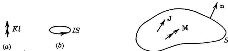
FIG. 3-3. These two sources radiate the same field if Kl = j\omega\mu IS . (a) Magnetic current element; (b) electric current loop.
